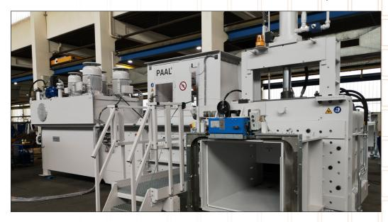
Kadant PAAL's HTR fully automatic, high-compression two-ram baler is a multipurposed baler for compacting municipal solid waste (MSW); refuse derived fuel (RDF); recyclable material such as plastics, carton, and paper into high density bales. The HTR baler compresses material with pressing force of 120 to 200 tons in a closed press box providing maximum bale weights. Its tying system, attached separate from the compression process, prevents disturbance to operation due to contamination.
